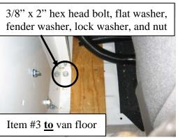
Secure the **Front Bulkhead**. Drill (2-one per-side) 3/8" holes through the frame, ½" plywood, and floor of vehicle Attach using 3/8" x 2" hex head bolt, flat washer, fender washer, and nut.
